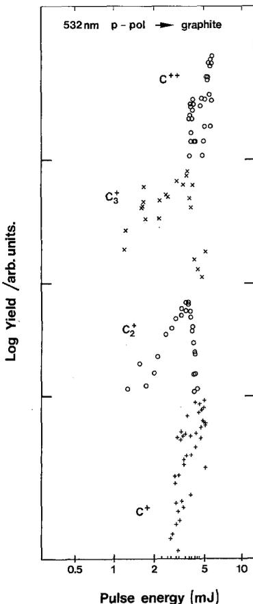
Fig. 2. Positive ion yields vs laser pulse energy as measured with the QMS (532 nm, p-polarized light). The  $C_2^+$ ,  $C_3^+$ , and  $C^{++}$  yields have been displaced vertically for clarity
