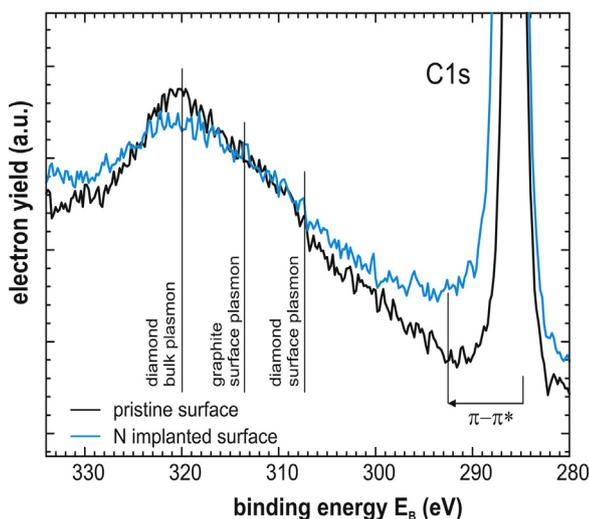
**Figure 4.** XPS detail spectrum in the vicinity of the C 1s peak. The black curve shows the result for the pristine surface while the blue curve represents the result after nitrogen implantation. (For interpretation of the references to colour in this figure legend, the reader is referred to the web version of this article.)
