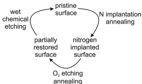
**Figure 1.** Cycle scheme for repetitive preparation of the diamond surface.
