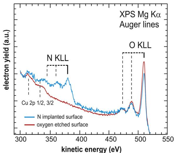
**Figure 3.** XPS Auger line analysis in the region of the N KLL and O KLL lines. The blue curve shows the result for the nitrogen implanted surface while the red curve demonstrates the complete removal of nitrogen after 27 h of etching in oxygen. The small Cu signal is ascribed to stray electrons emitted from parts made of copper at the nose of the X-ray source. (For interpretation of the references to colour in this figure legend, the reader is referred to the web version of this article.)
