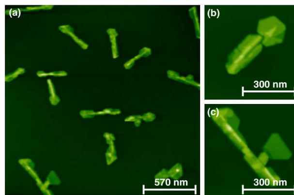
**Fig. 3.** (Color online) (a) Overview image of PTCDI islands covered by  $\text{C}_{60}$ .  $\text{C}_{60}$  molecules solely nucleate at the PTCDI islands and no isolated  $\text{C}_{60}$  islands are observed.  $\Delta f_{\text{set}} = -0.5$  Hz. (b) and (c) represent detail images demonstrating that  $\text{C}_{60}$  molecules also form larger patches attached to the elongated core.  $\Delta f_{\text{set}} = -3.5$  and  $-1.9$  Hz, respectively.
