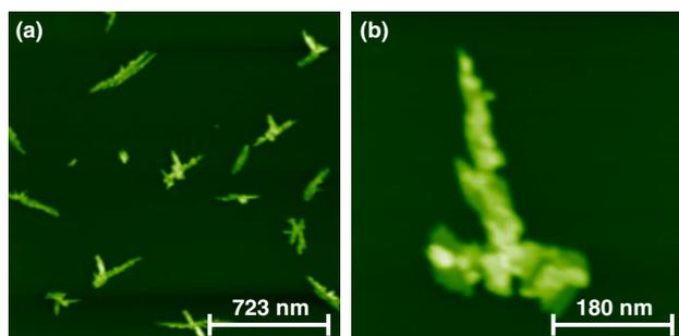
**Fig. 7.** (Color online) (a) Overview image of a  $\text{CaF}_2(111)$  sample after simultaneous deposition of PTCDI and  $\text{C}_{60}$ .  $\Delta f_{\text{set}} = -6.2$  Hz. (b) Zoom onto a characteristic island, exhibiting a more rough surface and irregular outer shape compared to the islands observed after sequential deposition.  $\Delta f_{\text{set}} = -1.3$  Hz.
