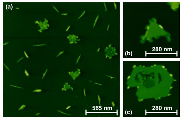
**Fig. 5.** (Color online) (a) Overview image of a sample initially covered with 0.1 ML of  $C_{60}$  and subsequent deposition of 0.1 ML of PTCDI. PTCDI molecules mainly arrange in needle-shaped islands and only few of them attach to the preexisting  $C_{60}$  islands.  $\Delta f_{\text{set}} = -1.0$  Hz. Frames (b) and (c) show details of  $C_{60}$  islands with attached PTCDI molecules.  $\Delta f_{\text{set}} = -10.0$  and  $-2.6$  Hz, respectively.
