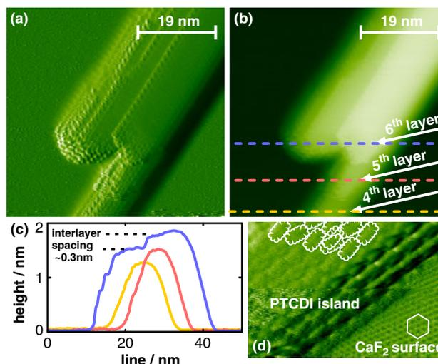
**Fig. 2.** (Color online) Zoom into the PTCDI island shown in Fig. 1(b). Both NC-AFM frequency shift (a) and topography (b) signals are shown.  $\Delta f_{\text{set}} = -10.0$  Hz. (c) Line profiles taken from the topography image as marked by the dashed lines in (b), revealing flat, stacked PTCDI layers. (d) Within the layers, the molecules arrange in a canted phase.  $\Delta f_{\text{set}} = -33.5$  Hz.
