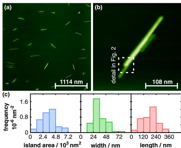
**Fig. 1.** (Color online) (a) NC-AFM overview image of PTCDI islands on  $\text{CaF}_2(111)$ . The image shows a large, atomically flat terrace with islands homogeneously distributed over the surface.  $\Delta f_{\text{set}} = -1.7$  Hz. (b) Individual island revealing an elongated shape and a stepped arrangement. The area enclosed by the square is shown in Fig. 2.  $\Delta f_{\text{set}} = -5.0$  Hz. (c) Statistical analysis from 60 PTCDI islands.
