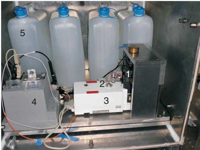
**Figure B1.** View on the environmentally controlled chamber housing the stiffness measurement system with removed front cover. The main components are (1) coarse and fine positioning units, (2) interaction zone with edge acting on the tip of the cantilever mounted on a balance stamp, (3) ultra-precision scale, (4) pressure gauge with control unit and (5) water container for temperature stabilization.
