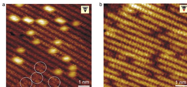
**Figure 2.** High-resolution nc-AFM images of the  $\text{TiO}_2(110)$  surface obtained with a negatively and positively terminated tip, respectively. The polarity of the tip is indicated by the triangular symbols. Image parameters: (a) size is  $10 \text{ nm} \times 10 \text{ nm}$ ,  $\Delta f = -14.4 \text{ Hz}$  and  $V_{cp} = +1.54 \text{ V}$ ; (b) size is  $7.3 \text{ nm} \times 9.3 \text{ nm}$ ,  $\Delta f = -36.1 \text{ Hz}$  and  $V_{cp} = +1.70 \text{ V}$ .
