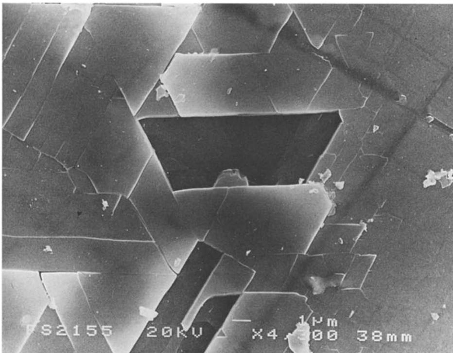
Fig. 4. SEM micrograph of surface damage resulting from single-shot irradiation at  $950 \text{ MW/cm}^2$ .
