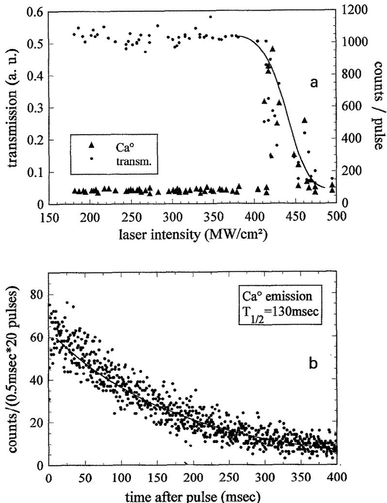
Fig. 3. Type 2 damage spot, irradiated with laser intensities below the ablation threshold. (a) Laser-intensity dependent  $\text{Ca}^0$  desorption yield and laser light transmission. (b) Time-of-flight spectrum of the delayed  $\text{Ca}^0$  emission signal integrated over 20 pulses in the vicinity of the intensity breakdown threshold.
