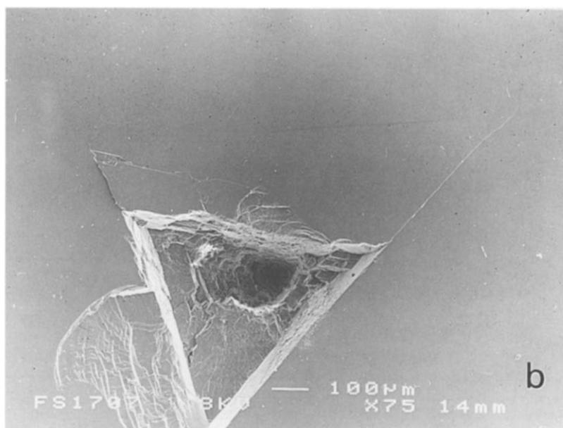
Fig. 1. Type 1 damage spot. (a) Laser-intensity dependent Ca<sup>0</sup> desorption yield and laser light transmission; (b) SEM micrograph of surface damage.
