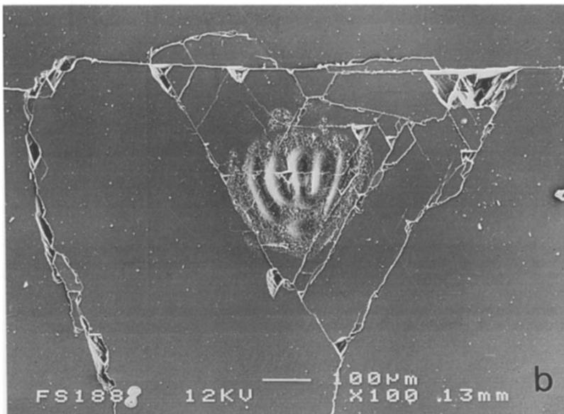
Fig. 2. Type 2 damage spot. (a) Laser-intensity dependent  $\text{Ca}^0$  desorption yield and laser light transmission; (b) SEM micrograph of surface damage.
