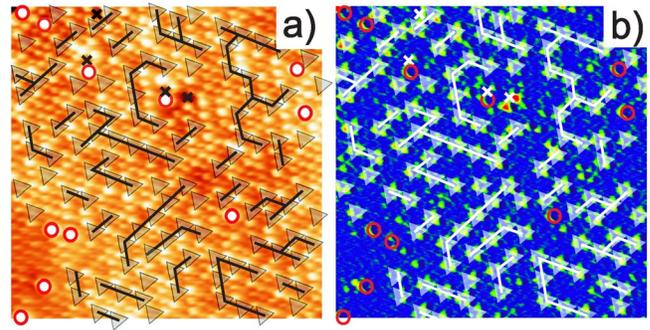
FIG. 3 (color online). Images shown in Figs. 2(a) and 2(b) where the association between the observed surface structure and the type of defect has been depicted. Triangles, crosses, and circles correspond to subsurface oxygen vacancies, surface oxygen vacancies, and hydroxide defects [10], respectively. The lines over both images highlight the arrangement observed for the subsurface oxygen vacancy structures.
