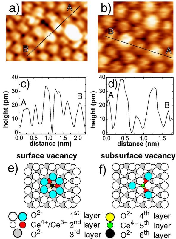
FIG. 1 (color online). DFM topographic images of a surface (a) and a subsurface (b) oxygen vacancy, together with the corresponding height profiles (c) and (d) and structural models (e) and (f), respectively. The protrusion at the right side of the surface oxygen vacancy (a) is ascribed to a hydroxide group substituting a surface oxygen [10]. The normalized frequency shift [23] image set points were  $-7.5 \text{ fN}\sqrt{m}$  for (a) and  $-2.9 \text{ fN}\sqrt{m}$  for (b), respectively [24].
