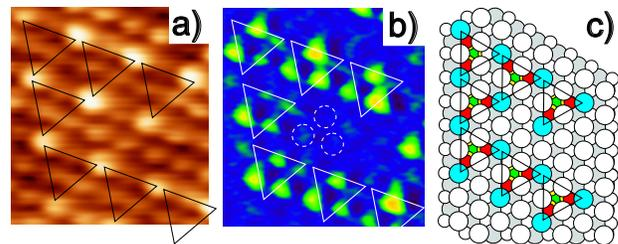
FIG. 4 (color online). Topography (a) and dissipation (b) images together with the corresponding schematic model (c) of the typical local ordering of subsurface oxygen vacancies observed in our images. The subsurface oxygen vacancy structures are highlighted by triangles. The dashed circles indicate a defect free surface area. The color coding of the model depicted in (c) is the same as in Fig. 1. The image set point was  $-2.9 \text{ fN}\sqrt{m}$ .
