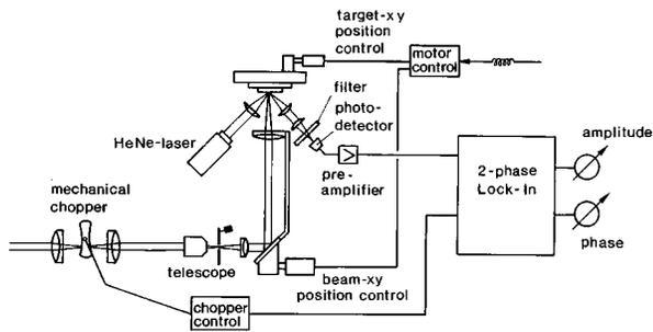
FIG. 1. Schematic view of the experimental setup used for thermoreflectance measurements.
