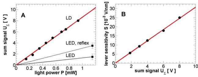
FIG. 4. (Color online) (a) Measured PSD sum signal  $U_{\Sigma}$  as a function of laser light power coupled into the FC/APC connector. (b) Optical lever sensitivity  $S$  as a function of  $U_{\Sigma}$ . Solid lines represent linear least-squares fits to the data. Dashed lines in (a) are a guide to the eye. LD: when the laser diode and uncoated cantilevers are used; LED: using LED with uncoated cantilevers; LED reflex: using LED and reflex coated cantilevers.
