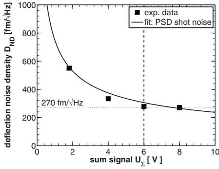
FIG. 6. Deflection noise density as a function of  $U_{\Sigma}$ . The solid line represents a least-squares fit to the experimental data according to Eq. (2). The dashed line corresponds to the sum signal typically used for NC-AFM experiments. A silicon cantilever (PPP-FM, Nanosensors)  $f_0=74\,720$  Hz,  $Q=69\,930$ , and  $k=2.8$  N/m was used.
