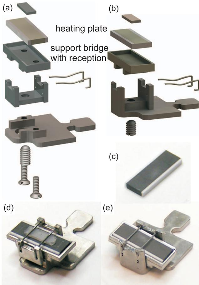
FIG. 3. Exploded drawing of a sample holder (a) in design I and (b) in design II remodeled for direct current heating. (c) Alumina heating plate with a tungsten strip directly fired to the substrate used as heating element. (d) Assembled direct current heating setup in design I with sample. (e) Assembled direct current heating setup in design II without sample.
