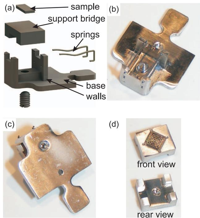
FIG. 2. Sample holder design II. (a) Exploded drawing of the sample holder. (b) Assembled base plate without support bridge. (c) Rear view showing the embedded fixation screw. (d) Support bridge with milled recess for precise placement of very small samples. A depression in the rear side acts as reception for the globular tip of the fixation screw.
