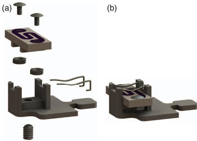
FIG. 4. (a) Exploded drawing of the sample holder designed for electrically conducting samples heated by a PBN heating element. (b) Illustration of the complete assembly without sample.
